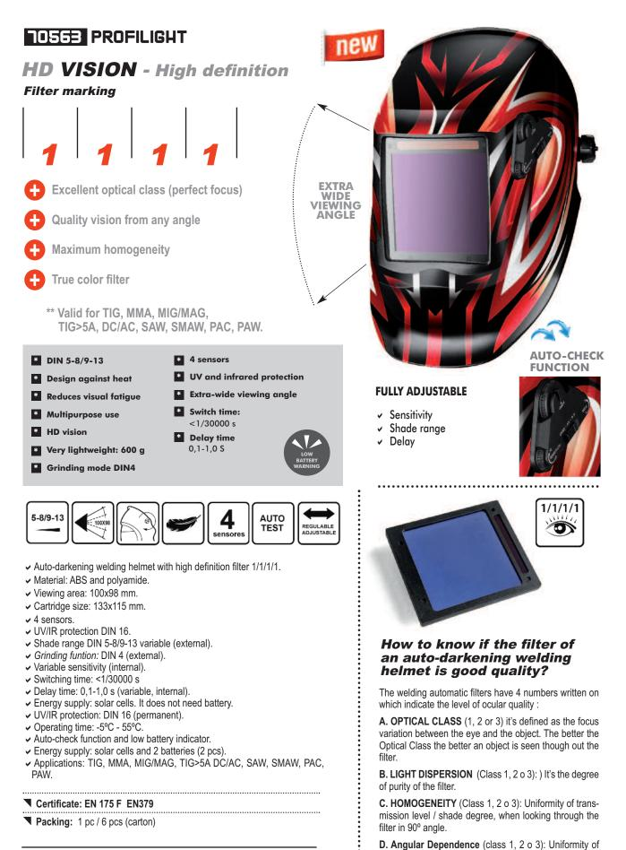
transmission level / shade degree when looking in different angles.
